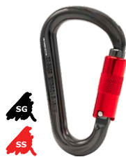
KH204 HMS Weight 93g (3oz) Gate Opening 22mm (7/8") MBS 27kN (6070lbf)
