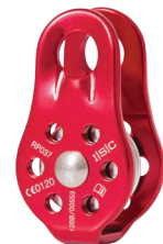
RP037 Micro Pulley Weight 90g (3oz) Max. Rope Diameter 13mm (1/2") MBS 28kN (6294lbf)
