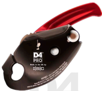
RP881 D4 Pro Descender No. of Persons 2 Rope Diameter Range 10.5mm - 11.5mm (7/16") WLL 240kg (529lb) Panic Brake No
