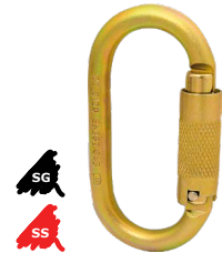
KL311 Oval Weight 188g (6.7oz) Gate Opening 18mm (5/8") MBS 25kN (5620lbf)
