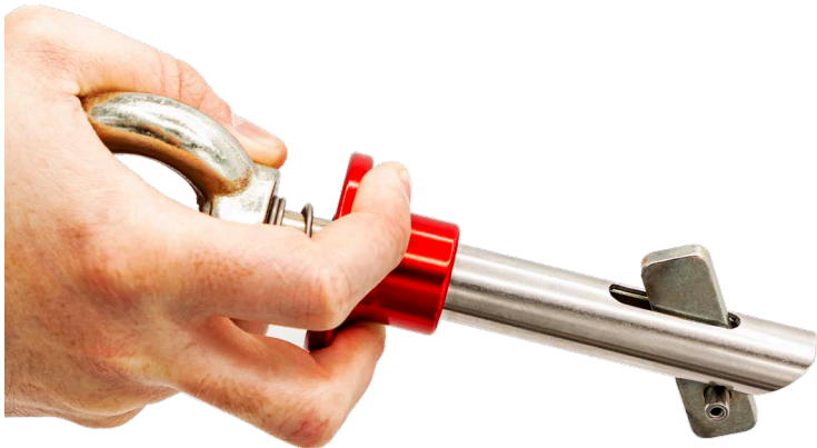
GG101 Girder Grip Weight 550g (19oz) MBS 28kN (6294lbf) Maximum Working Length 37mm (1 7/16")
