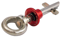
GG101 Girder Grip Weight 550g (19oz) MBS 28kN (6294lbf) Maximum Working Length 37mm (1 7/16")
