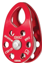
RP012 Small Single Pulley Weight 87g (3oz) Max. Rope Diameter 13mm (1/2") MBS 36kN (8093lbf)
