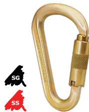
KH212 HMS Karabiner Weight 276g (10oz) Gate Opening 23mm (1") MBS 50kN (11240lbf)
