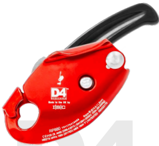
RP880 D4 Descender No. of Persons 2 Rope Diameter Range 10.5mm - 11.5mm (7/16") WLL 240kg (529lb) Panic Brake Yes
