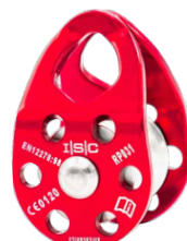
RP031 Double Re-direct Pulley Weight 124g (4oz) Max. Rope Diameter 13mm (1/2") MBS 30kN (6744lbf)
