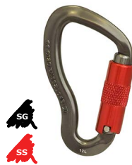
KH453 Gator Weight 46g (2oz) Gate Opening 15mm (5/8") MBS 25kN (5620lbf)
